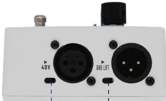
Slide right to engage **48V** phantom power for condenser microphones
